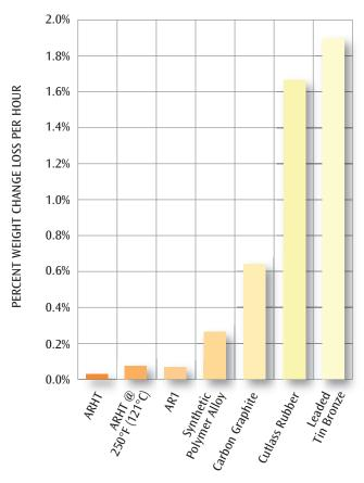
Note: Bearings made from each of the materials (size: 2 in. x 1.5 in. x 1.5 in./ 5.1 cm x 3.8 cm x 3.8 cm) were tested at 900 rpm under 25 psi (0.17 MPa). The run time of the test was eight hours. The test was conducted on 300 series SS shaft, in 95 percent water and 5 percent silica sand. All materials were tested at 70°F (20°C). Additionally, ARHT was tested at 250°F (120°C) in ethylene glycol.
